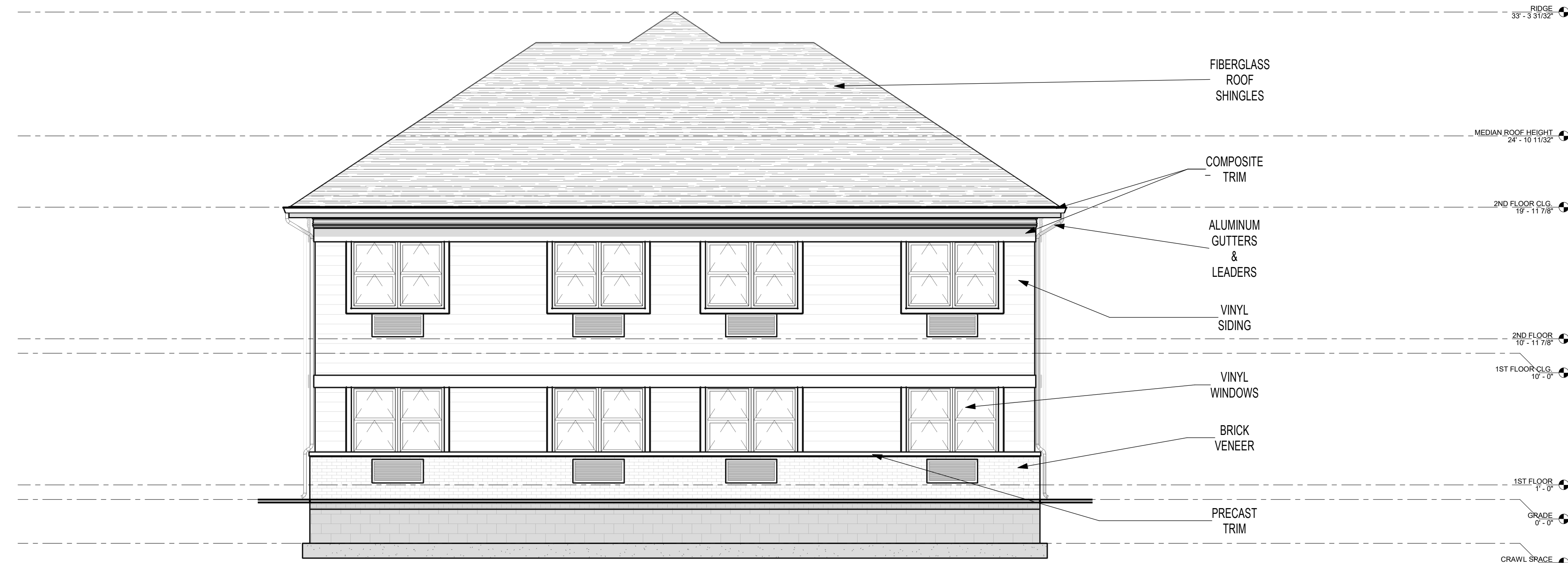
1 NORTH ELEVATION SCALE: 3/16" = 1'-0"
